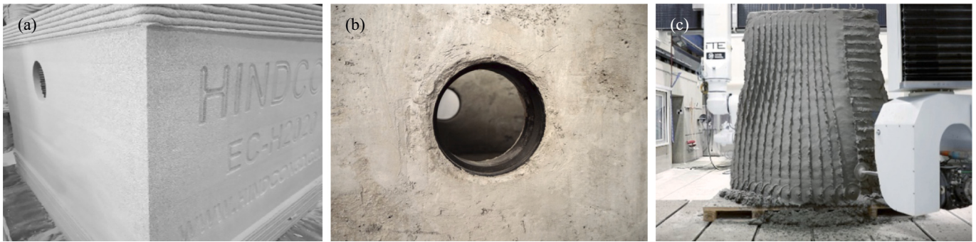
Fig. B.3. Exemplary applications of surface post-processing: (a) 3D concrete printed element with a partially milled surface [68]; (b) trowelled surface with insert of an element 3D printed with sprayed concrete [73]; (c) surface post-processing with a milling tool [71].
