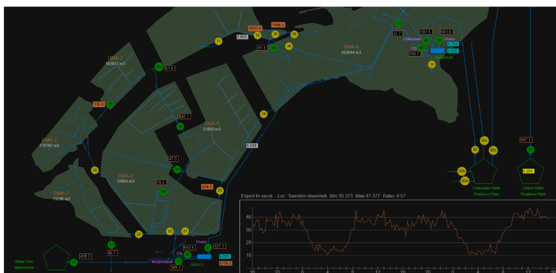
Figure 48: SCADA flow monitoring panel for Batumi's DMA inlets
