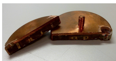
(a) Base with the copper cap and filled of epoxy
