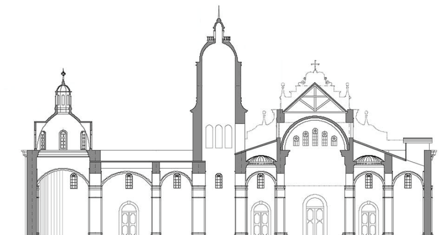
Figure 7. Ambato Matriz Church. Graphic restitution of the transverse section at the foot of the temple and transversal chapel.
