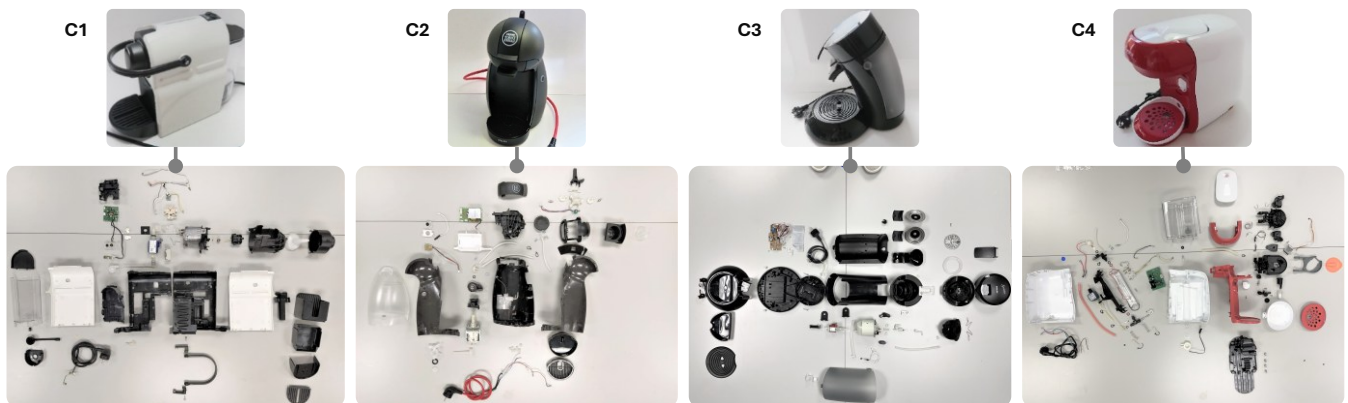
FIGURE III.5 CAPSULE COFFEE MACHINES FOR THE CASE STUDY AND THEIR DISASSEMBLY.
