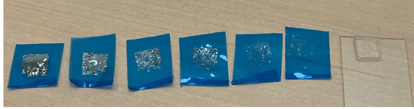
Figure 6.13: Tape-to-tape mechanical exfoliation of bulk HOPG.
