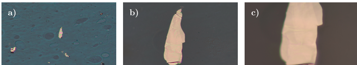
Figure 6.34: Optical micrographs ( 10\times , 50\times , 100\times ) of the selected few-layer graphene candidate supported on adhesive tape.
