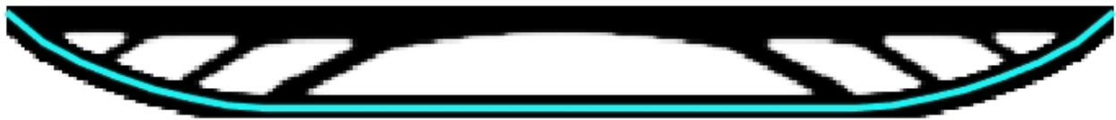
Figure 12: Results of the topology optimization procedure for a single-span beam subjected to a uniform load. Black represents concrete; white represents void; cyan represents the tendon [36].
