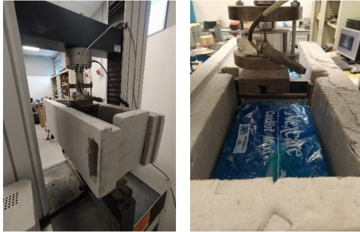
Figure 44. Insulation system used during 3PBTs.
