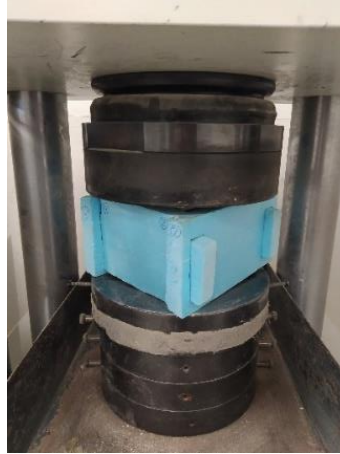
Figure 43. Insulation system used during compression test.
