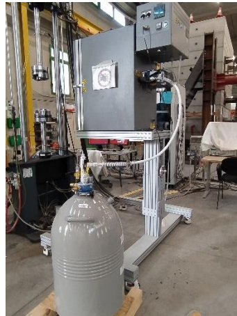
Figure 41. Set-up for direct tensile test on fibers at low temperatures. Nitrogen liquid incorporated to the MTS 651 environmental chamber.
