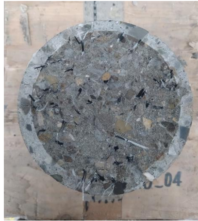
Figure 74. Example of a cylinder with a non-homogeneous distribution of fiber on its fracture surface.
