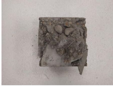
Figure 59. Debonded paste aggregate at 60 °C.
