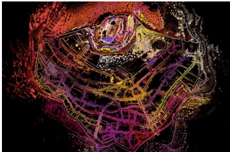
Fig. 4- Integration of the database obtained from TLS and MLS scans of the Morella city centre and Castle. Each colour highlights a different scan, highlighting the large number of scans taken to document the fortified systems of the walls and castle. Graphic elaboration by Francesca Picchio, Francesca Galasso, 2024.
