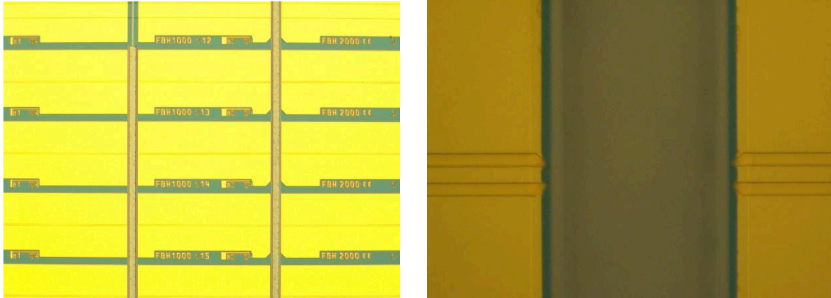
Figure 4.20. K1-Layer optical inspection of wafer 1 after lithography.
