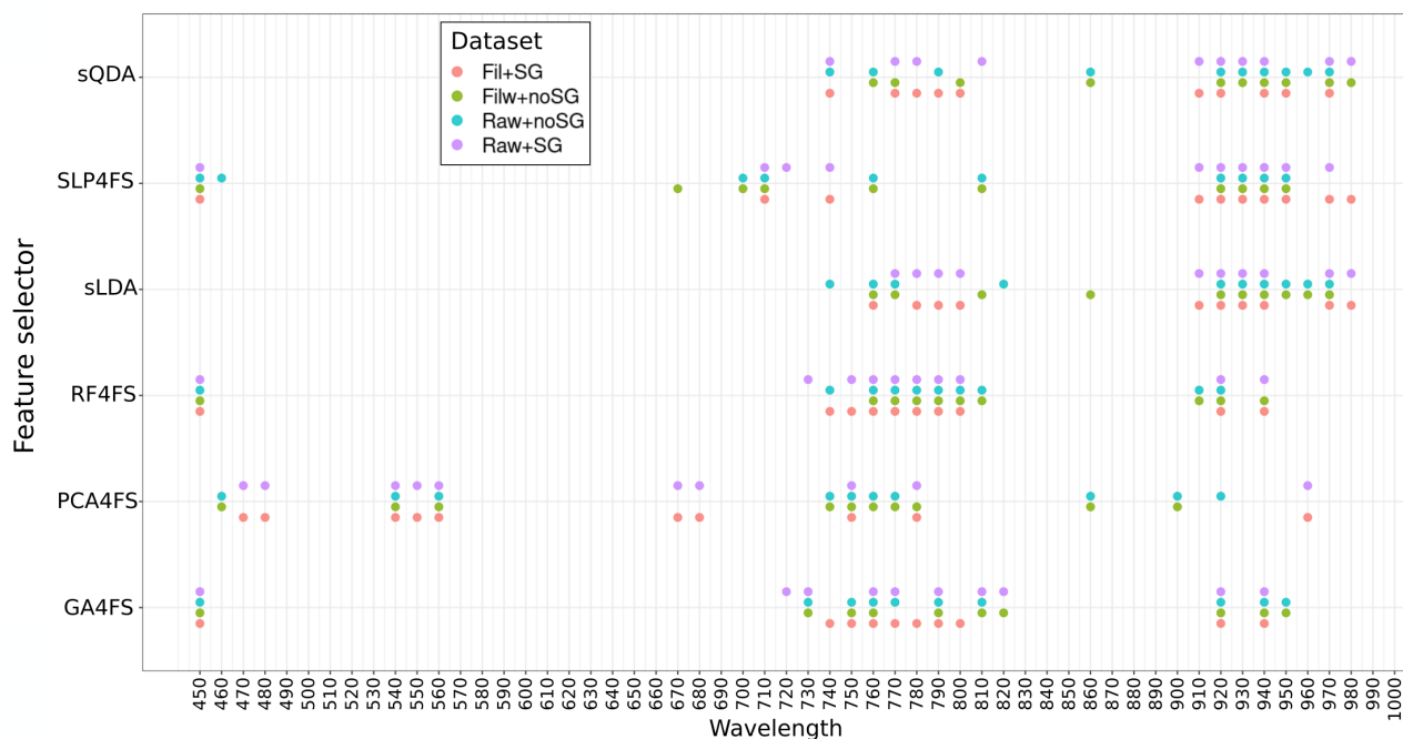
Figure 6-49. Group of wavelengths selected by the feature selectors, per defined dataset, for the e4-kt assay of the ‘Keitt’ mango fruit cultivar
