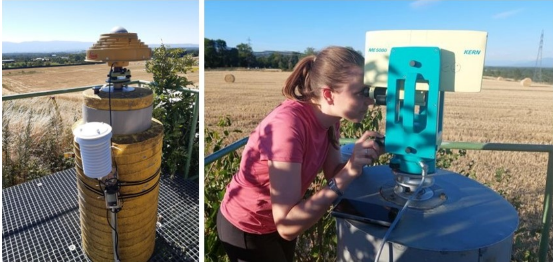
Figure 9: CERN pillar set-up (left), Mekometer measurements (right)
