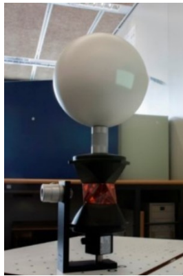
Figure 35: Target point consisting on reflector and sphere
