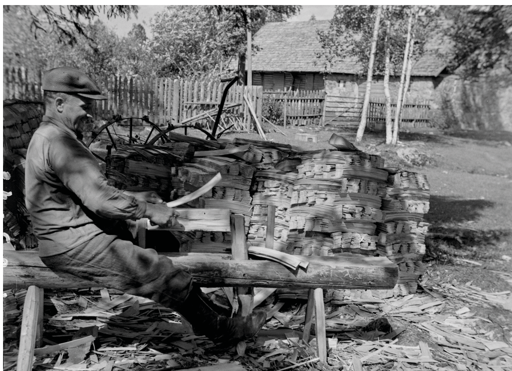
Fig 4 – A special splitting bench was used to split pilbas shingles by hand with a drawknife (Estonian National Museum, 1947).
