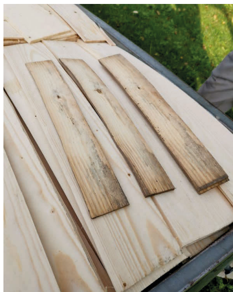
Fig. 6 – Hand-split thin pilbas shingles compared to mechanically produced laast shingles (Lutsepp, 2019).
