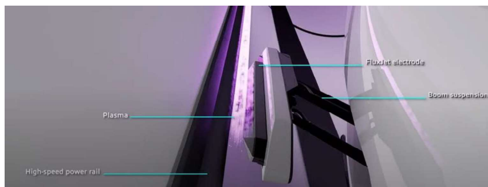
Figure 14: Primary Power Pickup system of the FluxJet, source: TransPod Inc. 2024
