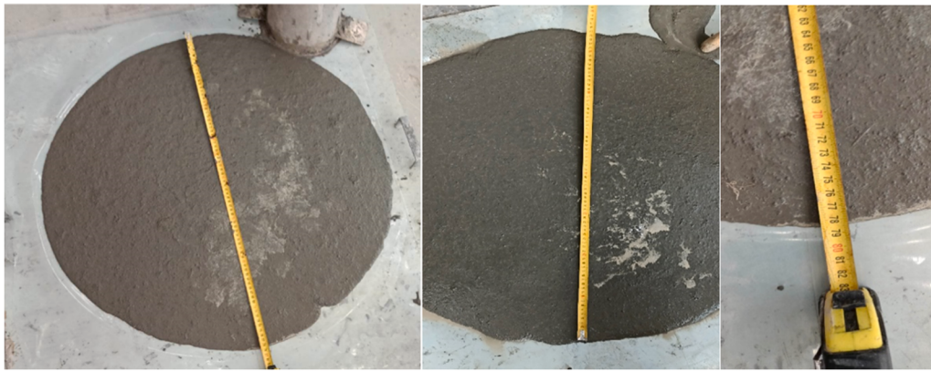
Fig. 16. Slump flow tests images of investigated UHPC mixes highlighting self-levelling behavior.
