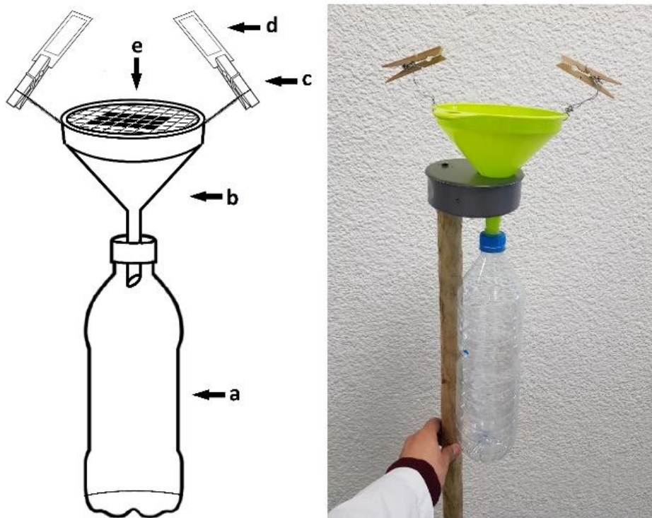
Figure 3.1 Schematic representation (left) and real (right) of the spore trap that was used to study the dynamics of Diaporthe amygdali conidia released from pieces of naturally infected almond shoots with cankers. The spore trap is composed of: (a) removable plastic bottle, (b) plastic funnel, (c) wooden clip anchored to the sides of the funnel, (d) glass microscope slides with silicone-coated tape and (e) inoculum source.
