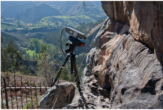
Fig. 8 View of the Specim V10E spectrograph scanning the lower bench of the site
