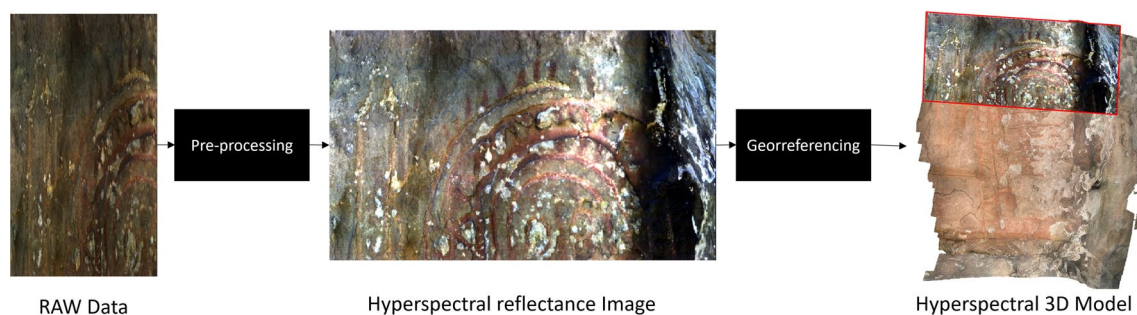
Fig. 21 Parallax process between radiometric data and geometric models
