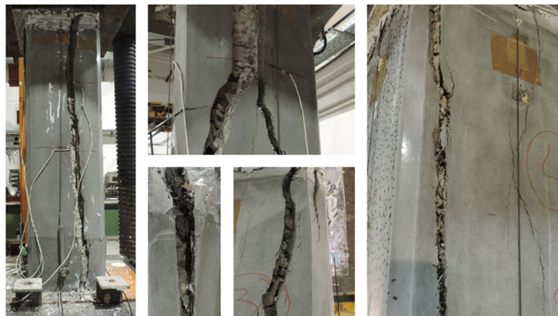
Figure 15. Details of the failure of square columns.
