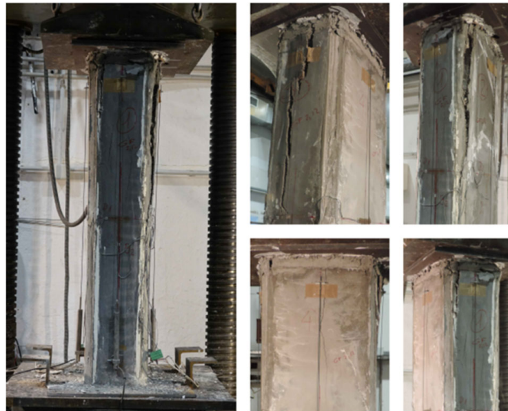
Figure 17. Details of the failure of rectangular columns with b/h = 2 .
