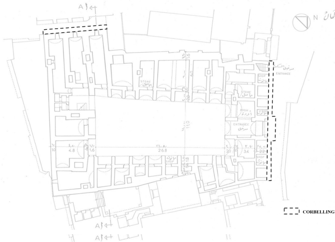
Fig. 11. Corbelled upper stories of Wekalet Bazaraa illustrating the façade overhang as a shaded transitional threshold between street and shop. Source: Base archival material from the Saleh Lamei Collection (1987), courtesy of the Rare Books and Special Collections Library, The American University in Cairo, used with permission; analytical reconstruction and diagramming by the author.
