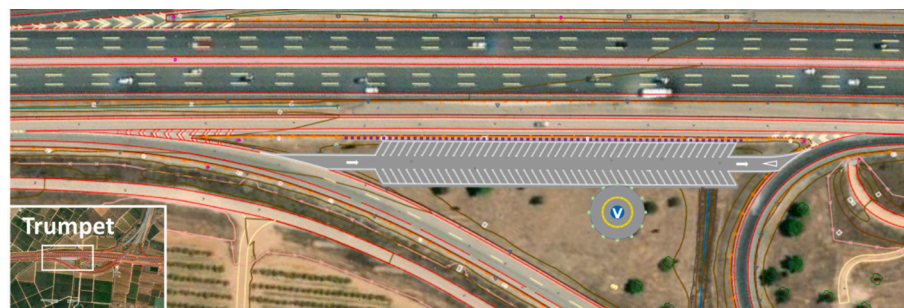
Fig. 14. Safe Harbor located in a trumpet.
