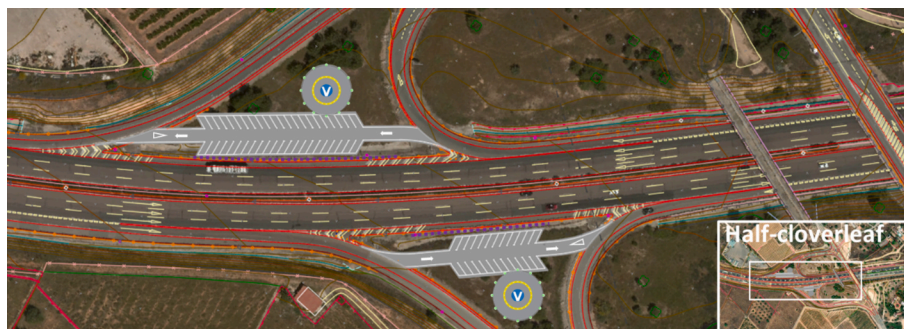
Fig. 13. Safe Harbor located in a half-cloverleaf.
