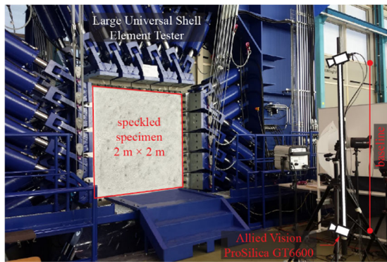
Figure 2. Digital image correlation setup in the Large Universal Shell Element Tester used for the uncertainty quantification in Section 3.1.3.
