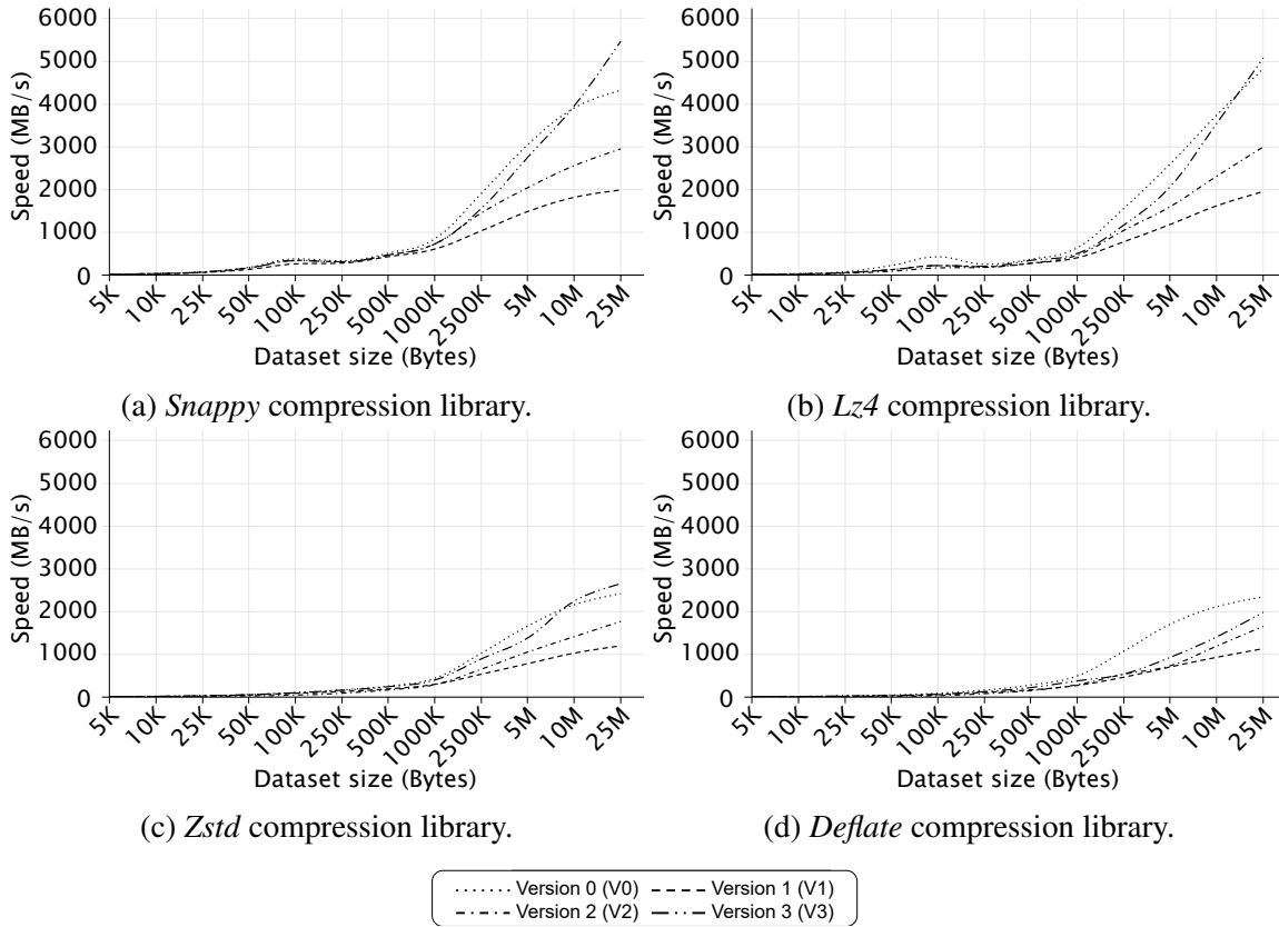
Figure 5.16: Comparison of the compression and decompression speed achieved by Version 0 (V0), Version 1 (V1), Version 2 (V2), and Version 3 (V3).
