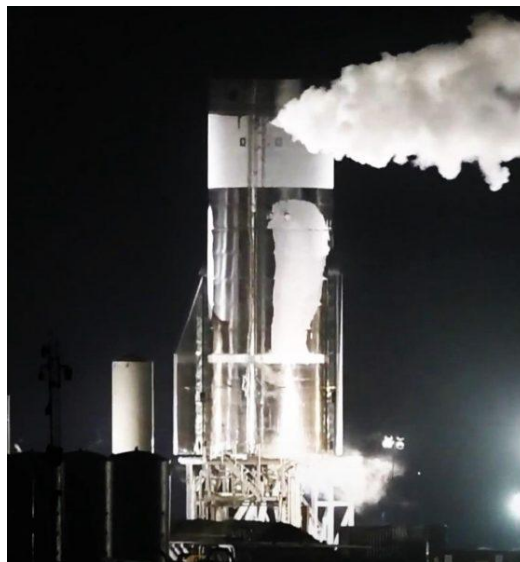
Figura 21: Proof test de la Starship (SpaceX)
