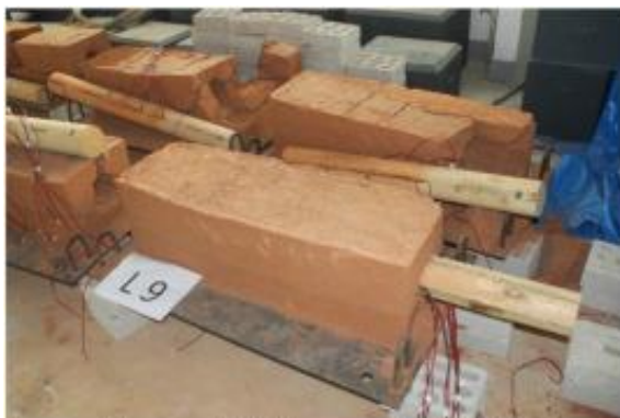
(a) overall failure mode of joint
