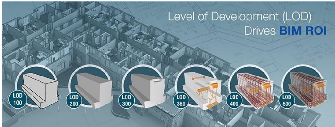
Ilustración 6. BIM Level of Development (LOD).
