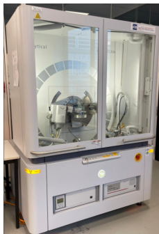
Figure 3.9: Malvern Panalytical-Empryeon XRD equipment.
