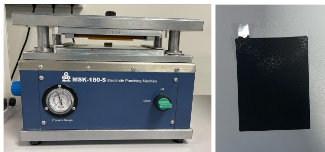
Figure 3.3: Punching machine used for cutting and cathode in its final shape after the process necessary for the pouch cell.
