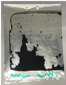
Figure 4.2: Brittleness of the 90/7/3 low-loading cathode.
