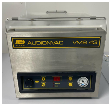
Figure 3.8: Device used for sealing the pouch cells (Audionvac VMS 43).
