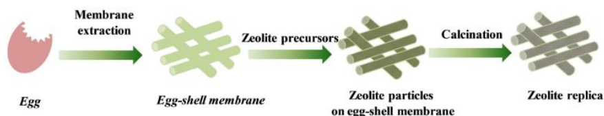
Figure 1.11. Egg-shell directed synthesis of micro-macroporous MFI type membrane. Obtained from Srivasta et al 114 .
