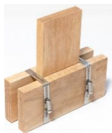
Fig.82 Fastening demonstration detail [Project (Un)Build, 2025]
