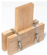
Fig.82 Fastening demonstration detail [Project (Un)Build, 2025]
