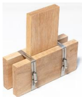
Fig.82 Fastening demonstration detail [Project (Un)Build, 2025]
