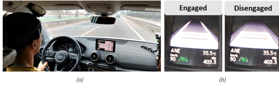
Fig. 2. Data collection: (a) Vehicle instrumentation and (b) status of the automated driving system.
