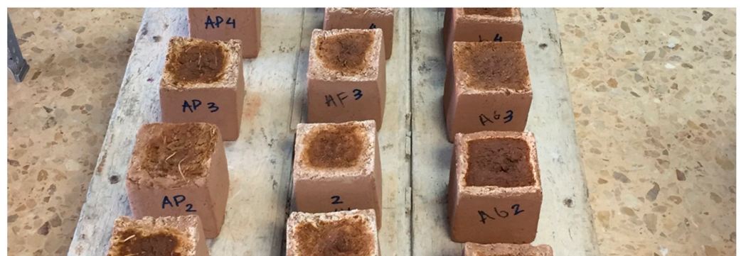
Figure 10. Adobe test specimens following the surface water erosion test by controlled water drop or dry test, showing the formation of localised cavities on the exposed face.
