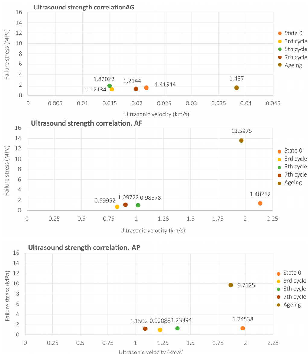
Figure 14. Correlation between ultrasonic velocity and tensile strength of coarse adobe (AG), fine adobe (AF), and adobe with fibres (AP) in different wetting–drying cycles.
