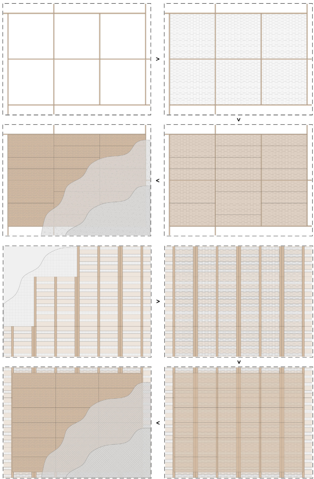
Figure 16 | Alternatives for constructing a roof using PO: square colombage or inverted pallets on a waterproof sheet after forming slopes; placement of fibers; closure of the “bousillage box” with wooden boards; coating with lime and clay or geotextile and gravel (credit: author, 2025).
