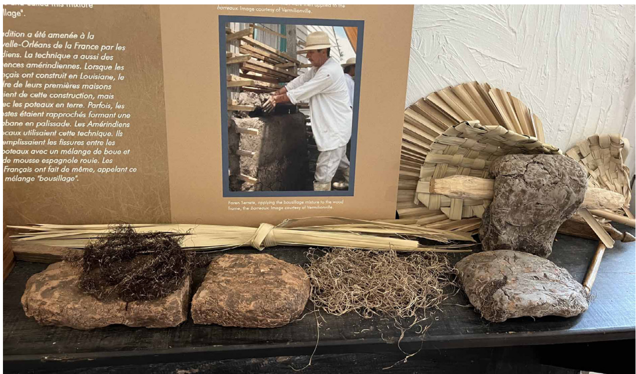
Figure 9 | Samples of cured and dried SM fibers, with the respective mud mixtures for bousillage (credit: author, 2023)
