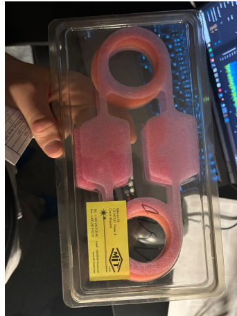
(b) CWDM filter (1311 nm).
