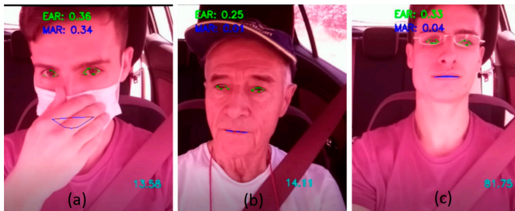
Figure 19. Correct operation with the use of accessories: (a) mask, (b) cap, (c) glasses.
