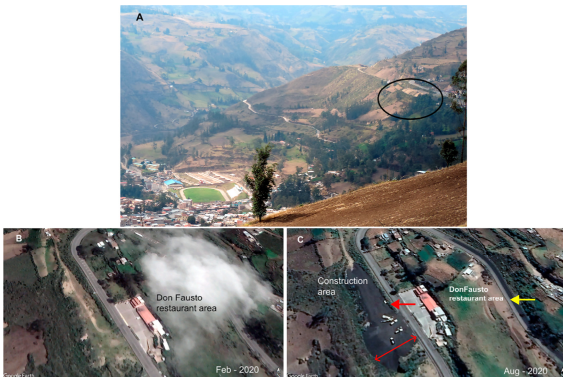
Figure 6. (A) A broad view of the location of the anthropic landfill between the Casual and Nuevo Alausí neighborhoods (black oval). That anthropogenic deposit was located in the head of the area of the landslide (the Don Fausto restaurant is to the right of the oval). The slide materials would cover the football field in the picture’s left corner. (B) On 4 February 2020, it can be noted that no anthropic landfill was in front of the restaurant, as shown in the picture [17]. (C) On 29 August 2020, it can be seen in the image that black landfill was deposited in the area (red arrow) where some earth machinery was working [17]. The yellow arrow shows where the cut-and-fill material was deposited from the E-35 Road construction, and the double arrow line shows a 55 m length.
