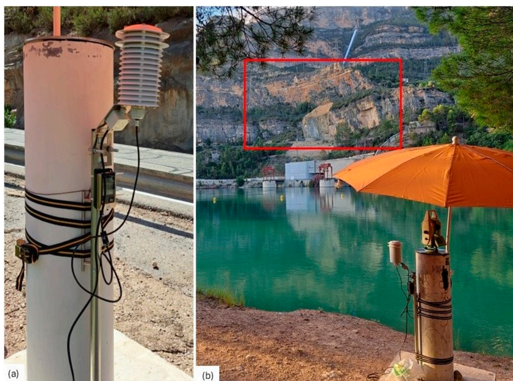
Figure 5. (a) Detail of a meteorological sensor with self-ventilated shelter. (b) Total station and meteorological sensor in point 8009 in the June 2024 campaign. The area of target points is marked in red.
