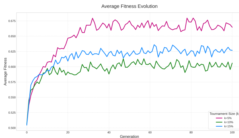
Figure 5. Evolution of average population fitness over 100 generations. The plot compares the performance of three different tournament sizes ( k ): k = 5\% (pink), k = 10\% (green), and k = 15\% (blue).
