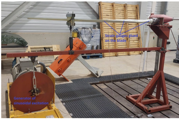
Fig. 7 Fatigue test setup for thermoplastic blade with horizontal crank and saddle load application at 1.44 m
