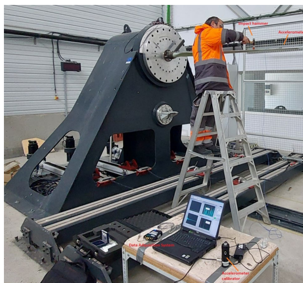
Fig. 5 Property test: measurement of natural frequencies
