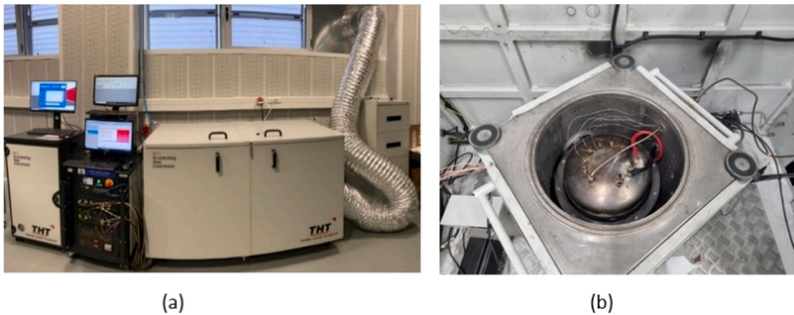
Fig. 1. Experimental Setup with the EV + ARC, (a): CMT-UPV battery lab, (b): the setup measurement system (b).
