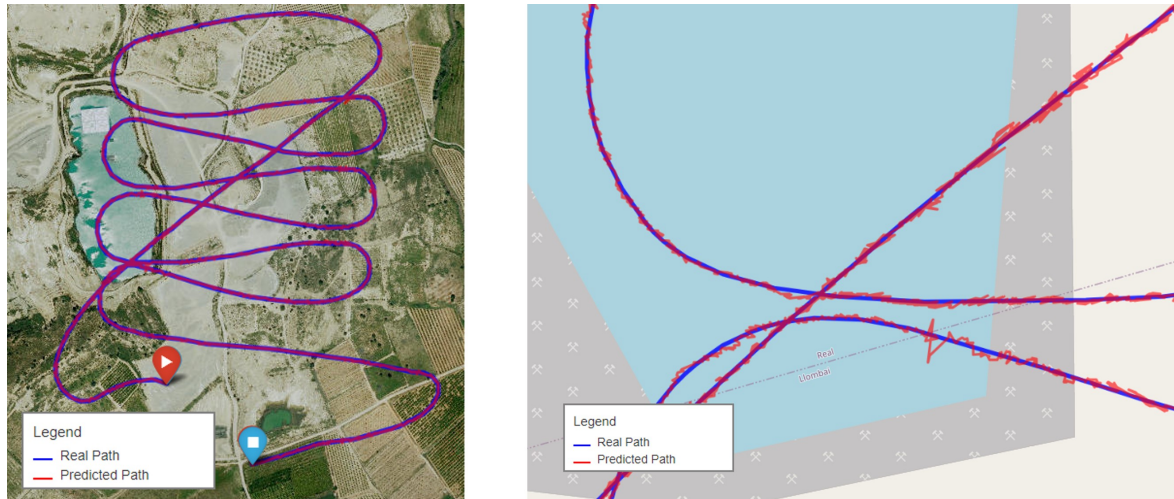
Figure 14. Predicted (red line) vs. real coordinates (blue line) obtained through the GPS predictor model (left) and detail of the predictions (right).
