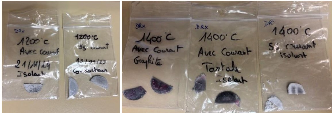
Figure 65. Samples sintered at 1200 °C and 1400 °C with and without current
