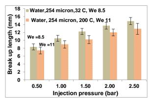
Figure 4a. Effect of injection pressure on the breakup length
