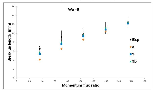
Figure 5b. Effect of momentum flux ratio on the breakup length (We =5). Experimental values are plotted along with the values predicted by equations (8), equation (9) and equation (9b)
