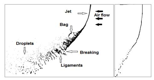
Figure 1. Typical jet in cross flow showing bag breakup and column breakup regimes (not to scale)
