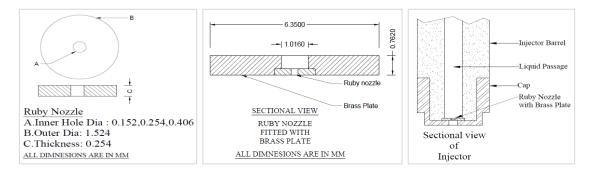
Figure 2b. Ruby Nozzle, Ruby nozzle fitted with brass plate and the Injector
