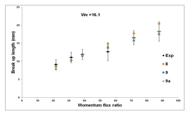
Figure 5a. Effect of momentum flux ratio on the breakup length (We =16). Experimental values are plotted along with the values predicted by equations (8), equation (9) and equation (9a)
