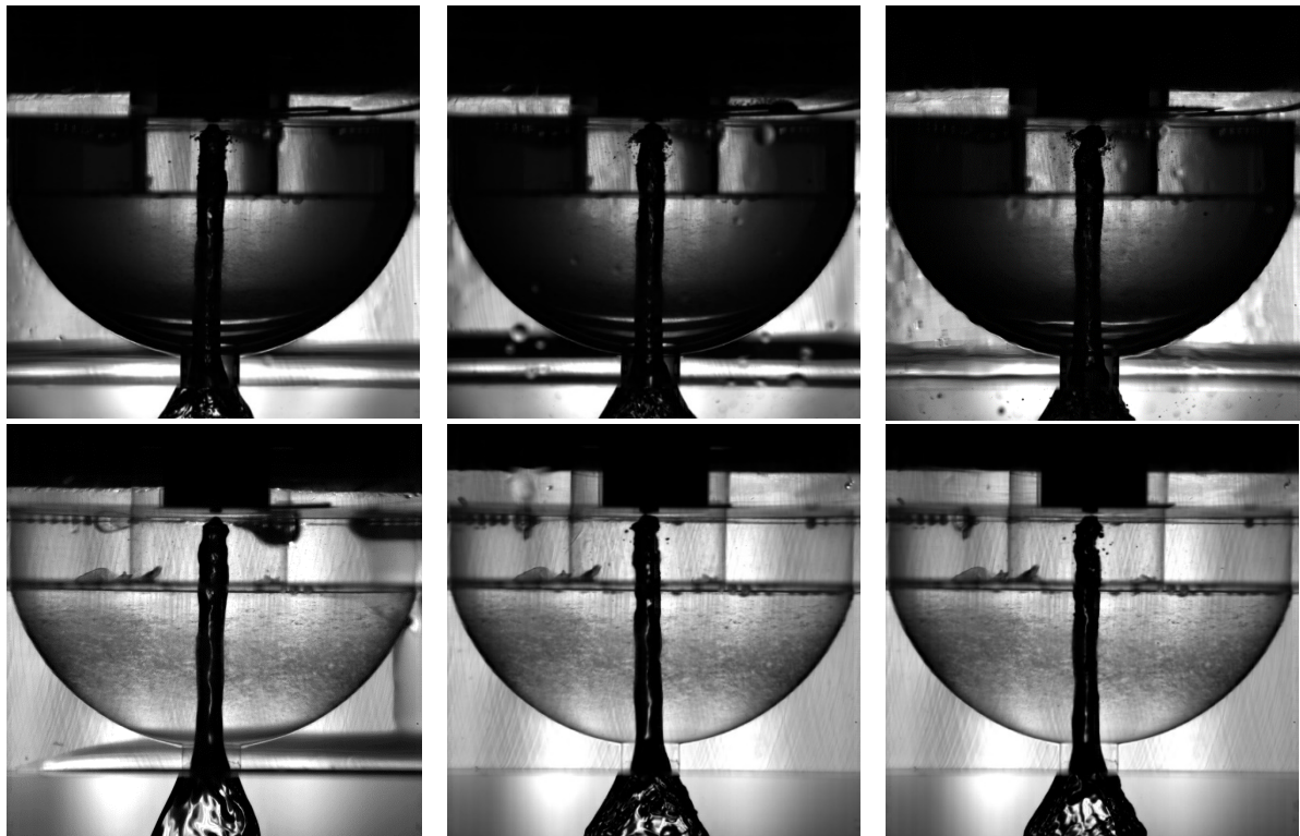
Figure 4. Simplex atomizer, Top: Kerosene, Bottom: P-cymene. From left: equivalent 0.5 MPa ( Re = 755 ), equivalent 1 MPa ( Re = 1021 ), equivalent 1.5 MPa ( Re = 1252 ).
