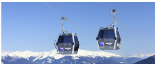
Figure 1: Self detachable aerial cableways. Suspended on a hauling and sustaining rope, the cabins need to face big stresses from inertial forces and additional wind loads.
