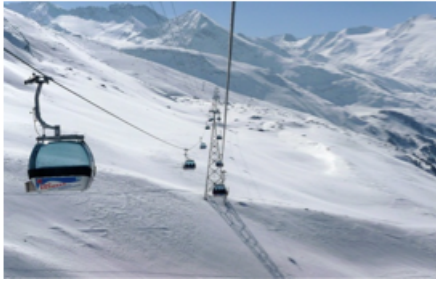
Figure 4: The researched case considers 5 cabins simultaneously on the same span. The distribution of the weight along the span is . therefore considered to be constant all along the span.
