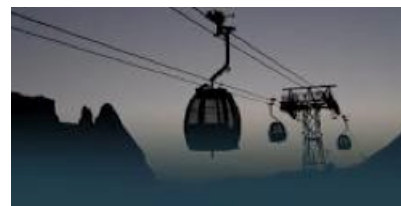
Figure 7: A quasi oval cabin, used in the skiing resort of Alpe di Siusi in Italy. These cabins have better aerodynamic performance. However, they don't let skiers to put their skies outside the cabin, as happens in the Sigma cabins.
