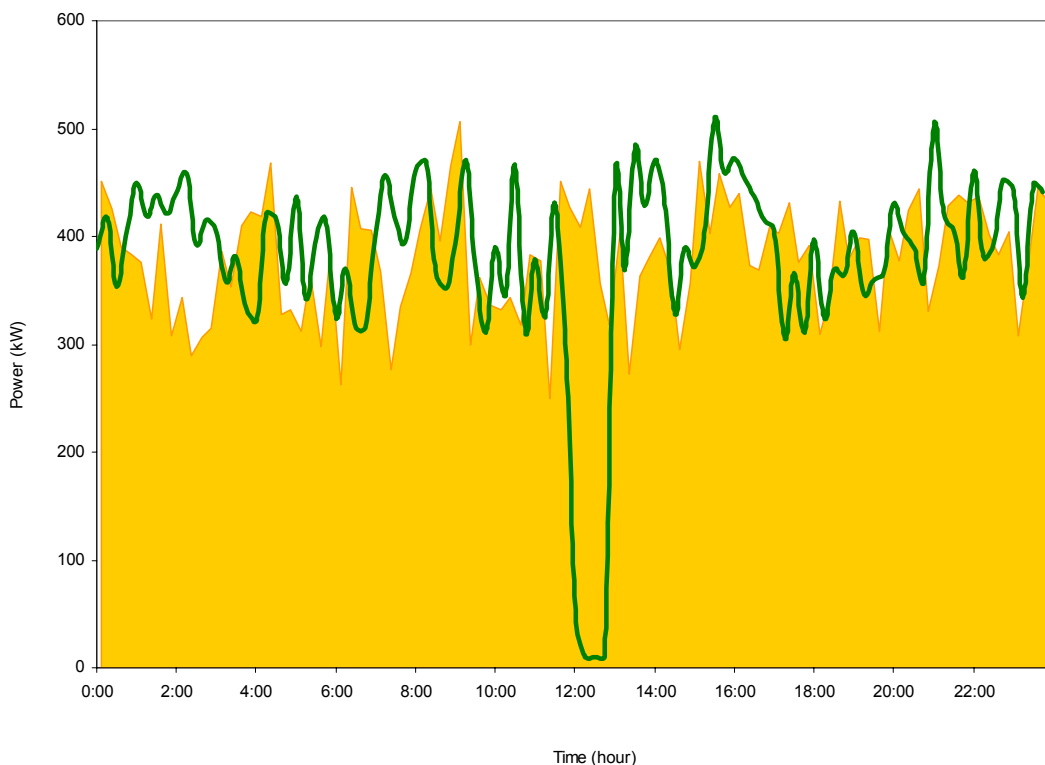
Figure 31. Pre-evaluation test performed in a cured ham factory This figure shows a comparison between the load curve of two consecutive working days where flexibility was (green line) and was not applied (orange area).
