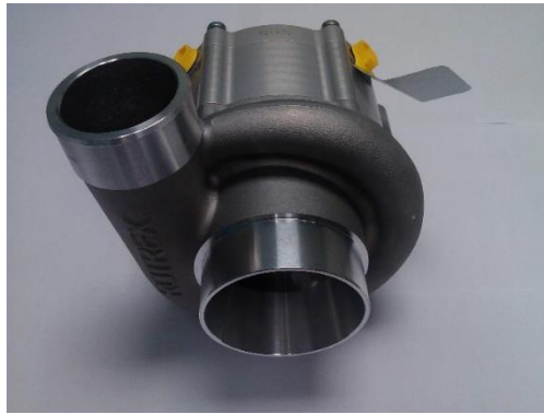
Figure 3.10 – Mechanical compressor Rotrex C38-92
