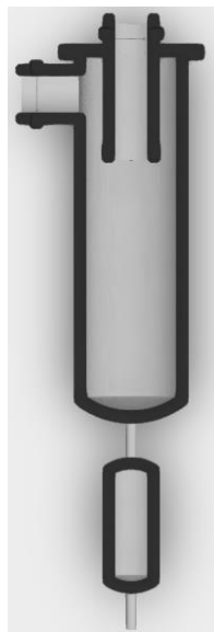
Figure 3.8 – Frontal section of the cyclonic separator
