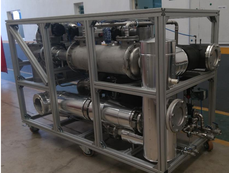
Figure 3.35 – Altitude simulator internal aspect
