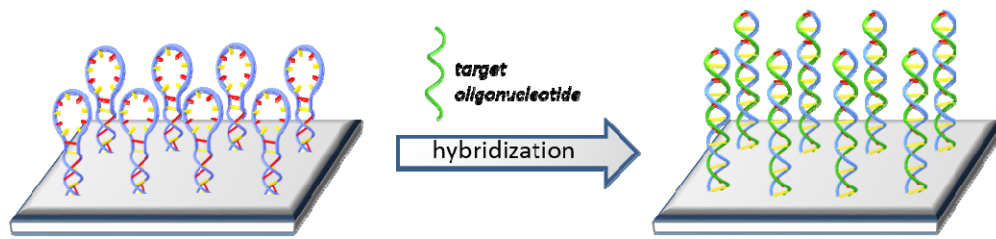
Fig. 3. Scheme of the hybridization event having the MBs immobilized on the surface of a photonic structure.
