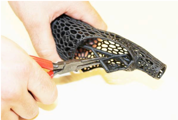
Figure 6. Manual removal of supports process.
