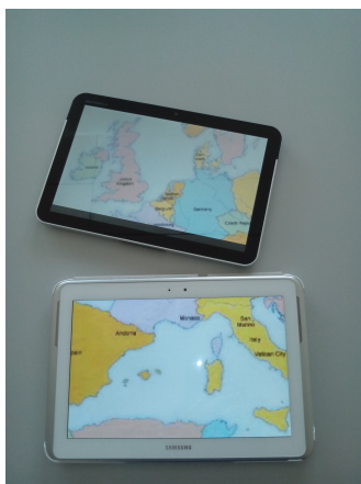
Figure 2.6: Example of MDE with homogeneous, planar, and irregular topology; and with extended-discontinuous logical view (extracted from Garcia-Sanjuan et al., 2016b).
