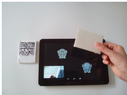
Figure 4.1: Interaction with MarkAirs to control the position of an element. On the left, the fiducial marker used.
