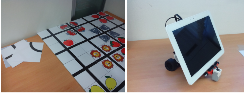
Figure 14.2: The tangible surface’s parts. On the left, the different tiles that compose the physical surface. On the right, the mobile robot that displays the digital content.
