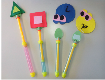
Figure 13.3: Extendable robot control paddles. From left to right: shift forward, stop, turn left, turn right.
