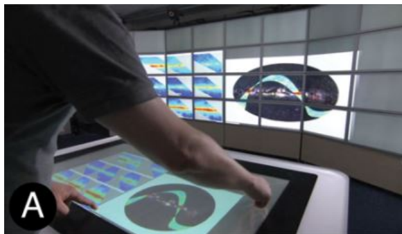
Figure 2.2: Example of MDE with heterogeneous, volumetric, regular, and perch topology; and with redundant logical view (extracted from Gjerlufsen et al., 2011).
