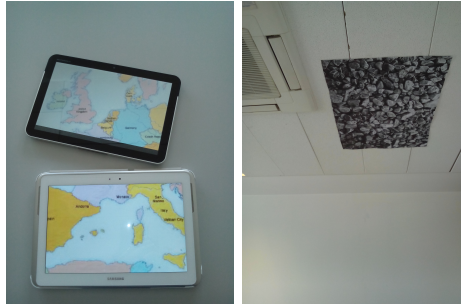
Figure 12.2: MDE using WeTab with several tablets on a table (left) and the reference image/marker on the ceiling (right).
