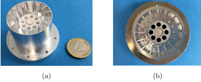
Fig. 6. Pictures of the fabricated radially corrugated horn antenna: (a) 3D view, and (b) upper view (RCW).
