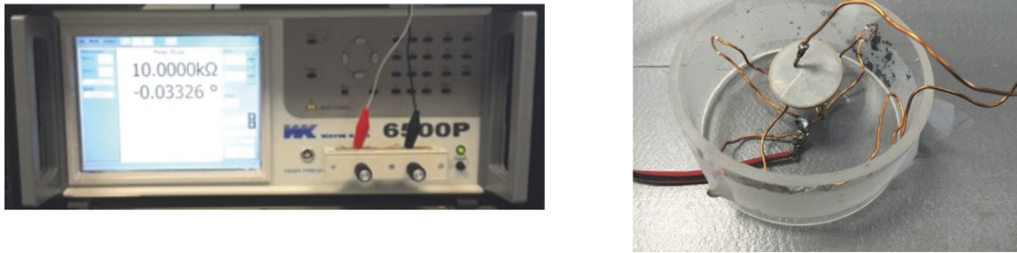
FIGURE 3: Experimental setup to measure the electrical impedance of the ceramics.
